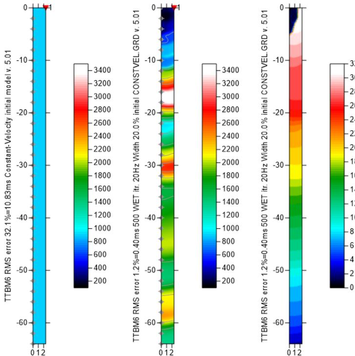
Fig. 13 : constant-velocity initial model (left). Steepest-Descent WET inversion after 500 iterations (center) with **discard WET smoothing** checked in *Model|WDVS Smoothing* (Fig. 11). Leave WDVS disabled.
