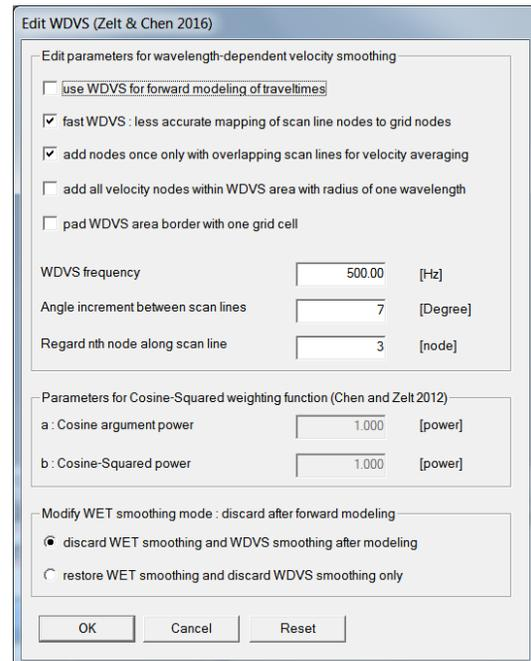
Fig. 11 : Model|WDVS Smoothing dialog. Click option **discard WET smoothing and WDVS smoothing after modeling**. Click OK.
