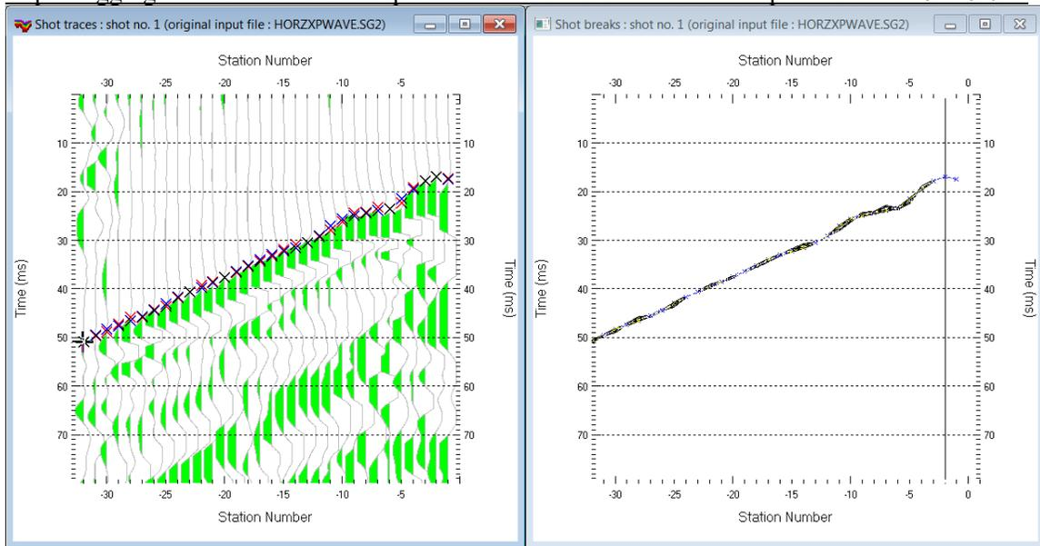
Fig. 1 : Left : Trace|Shot gather, right : Refractor|Shot breaks. Shows fit between picked times (solid curve, red crosses) and modeled times (dashed blue curve, blue crosses).
