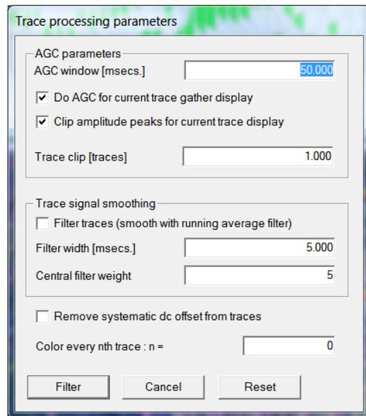
Fig. 9 : Trace processing parameters shown with **ALT+M**. Edit as shown and click *Filter* button.
