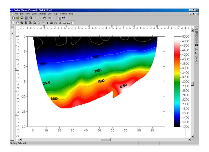
Please note the degree to which remaining Delta-t-V artefacts have been removed from the interpretation, by WET Tomography processing. Also, the "Dipping" model assumes a constant velocity overburden (1000 m/sec.) and a constant velocity basement (4000 m/sec.). In a more realistic model, the velocity in the overburden would increase with depth, e.g. linearly.
