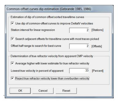
Edit these parameters for estimation of dip of common-offset sorted traveltime curves and for improved DeltatV velocity estimation :
