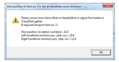
To **identify and fix bad shot positions** first configure your *Refractor*/*Shot breaks* display with Mapping menu items :
