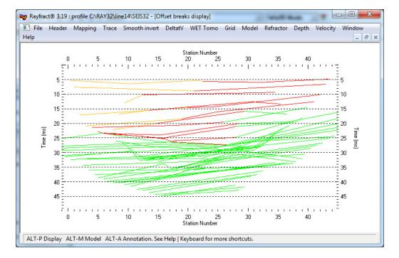
Common-offset traveltime curves displayed connect first breaks belonging to shot receiver pairs with constant unsigned offset along the profile. This kind of display lets you guess at refractor dip and shape even before doing time-to-depth conversion. Our Common-offset dip estimation dialog (available with our Pro license only) lets you estimate and use the dip of common-offset sorted traveltime curves to improve DeltatV inversion output in case of steeply dipping refractors.
