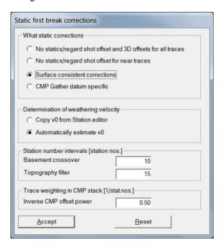
Edit these parameters, for correction of first breaks for undulating topography:
