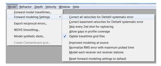
Select option *Model*|Forward modeling settings|Correct all velocities for DeltatV systematic error to reduce all grid node velocities as indicated in the Surfer® .GRD grid file by 10 percent before running the model through the raytracing algorithm.
