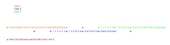
Geophones are spaced at 10-foot intervals and the shots are placed between the phones as indicated above. Each line will use 7 shot points at the same location as the overlapped spread. The overlapped geophones will occupy the same position for the next line. Length of line is 590 feet (59 spacings at 10' intervals) plus 20' for outside shots (each 10' off), for a total of 620'.
