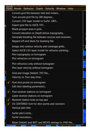
Then select the **DELTATV.TXT** or **MINVELO.TXT** as generated by our software. These .TXT files are located in your \RAY32\ profile subdirectory. Configure display and labeling of shot points and receivers on Surfer® tomogram plots with above *Grid menu* options.
