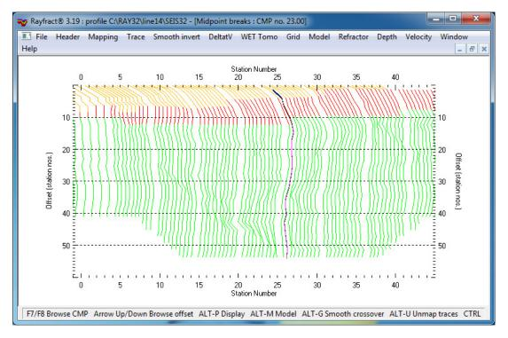
At each CMP (horizontal axis, in station numbers), a local coordinate system is appended, with its origin at that CMP. It has recording time as horizontal axis (not displayed; overlaps CMP station number axis) and unsigned shot point to receiver offset as vertical axis.
