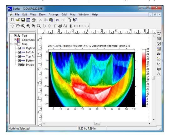
Select *Refractor/Shot breaks* to check match between modeled (dashed blue) and picked (solid grey or colored) traveltime curves :
