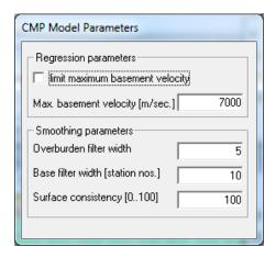
Parameters *limit maximum basement velocity* and *Maximum basement velocity* allow applying a low pass filter to CMP Intercept Time Refraction velocities estimated for the basement. When the estimated velocity at a station number exceeds the maximum velocity specified, no velocity and depth estimations are output for that station. Velocity and depth are
