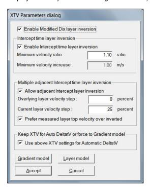
Our **XTV inversion implementation** assumes that apparent velocity increases with offset. So XTV triples are sorted by offset, for layer inversion as described here. (Winkelmann 1998) proposes the following XTV inversion algorithm:
