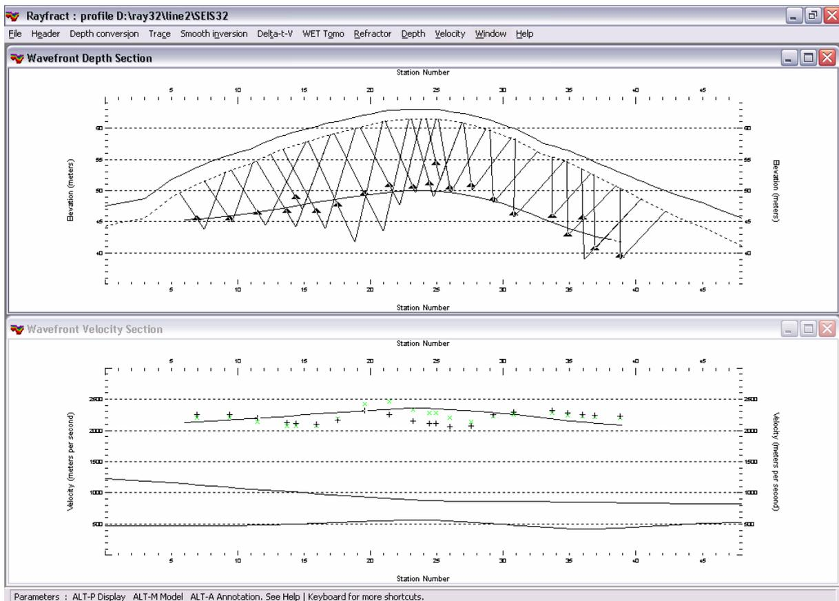
Conventional Wavefront method interpretation of LINE2. Modeling of two refractors.
