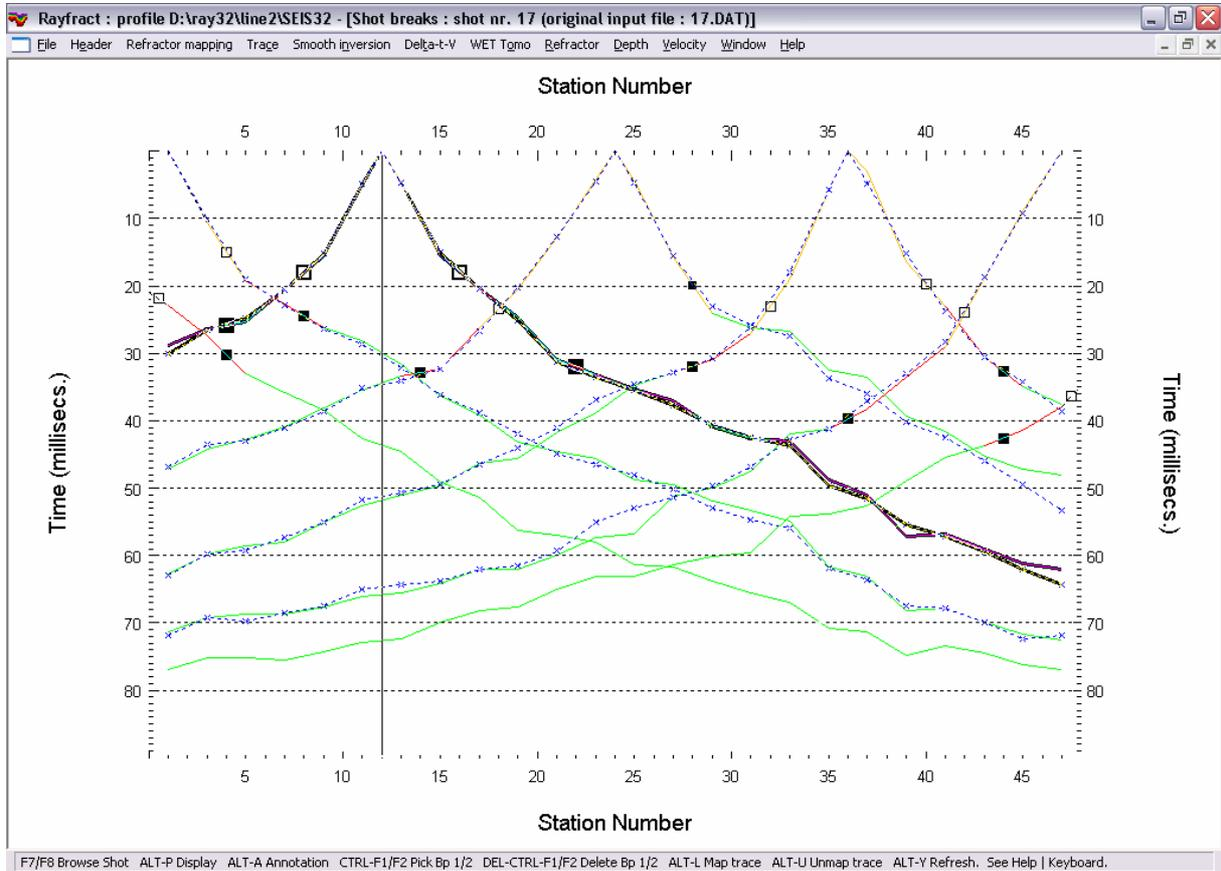
LINE2 fit of modeled (blue) to picked (colored) traveltime curves, after 100 WET iterations. Branch points (outlined squares: red refractor 1; black filled squares: green refractor 2) have been picked interactively; see manual chapter 1.8. Yellow traveltime curve segments are mapped to the weathering layer.
