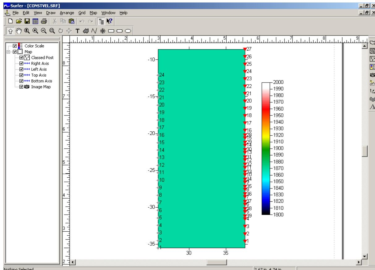
Constant-velocity initial model. Receivers 1 to 24 are in left hole, shots 1 to 39 in right hole.
