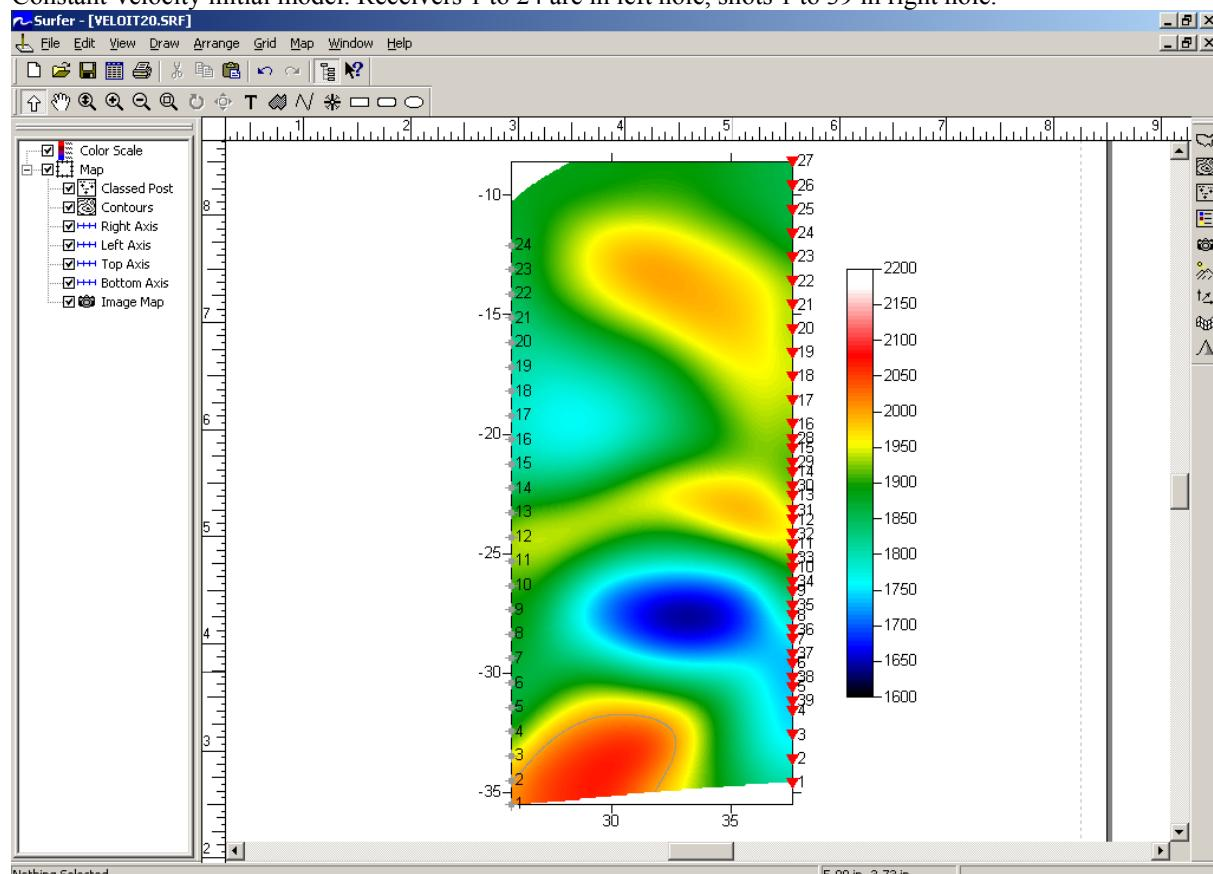
Smooth inversion output after 20 WET iterations. Compare with IGT crosshole tomography example (airport).
