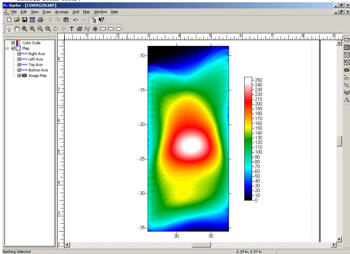
Coverage of IGTA13 grid cells with wavepaths, scaled with static Beydoun weighting .
