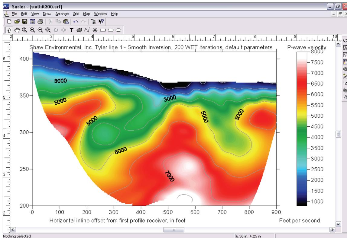
Smooth inversion : true 2D WET Tomography, 200 iterations. Default parameters. 1D gradient Delta-t-V initial model. Above output was generated with Rayfract™ version 2.62. For an interpretation of the same data set with GeoTomo LLC software, see Fig. 9 on page 341 in [Thomas L. Dobecki and Sam B. Upchurch 2006. Geophysical applications to detect sinkholes and ground subsidence. The Leading Edge. Volume 25, Issue 3, pp. 336-341 \(March 2006\).](#)
