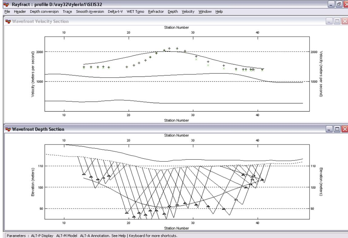
Wavefront interpretation. Station spacing is 20 feet (6 m). Basement elevation at station 20 (horizontal inline offset of 400 feet) is about 280 feet (85 m), with estimated velocity of 5,000 feet/sec. (1,500 m/sec). This nicely agrees with the Smooth inversion output, as shown below.
