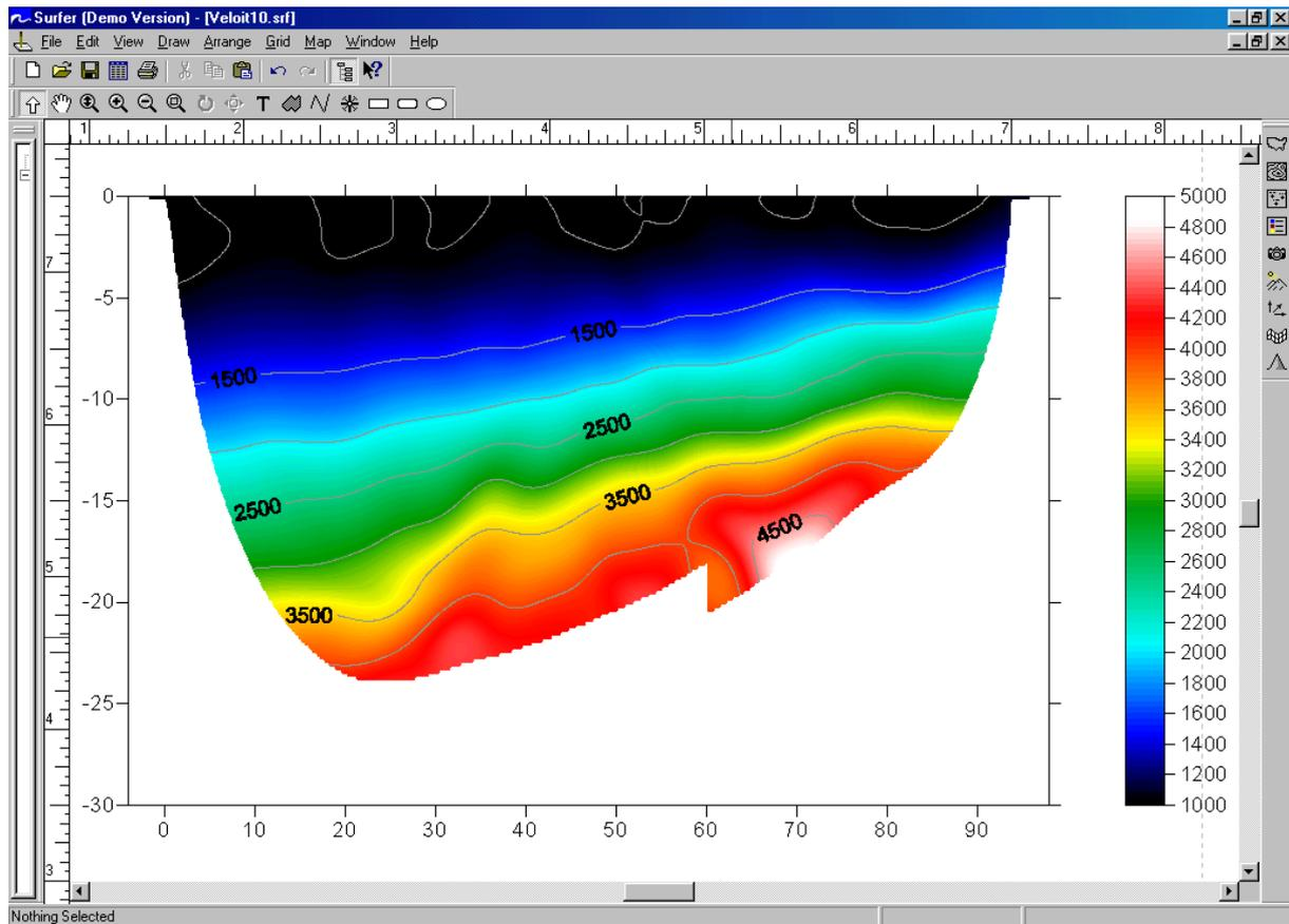
Please note the degree to which remaining Delta-t-V artefacts have been removed from the interpretation, by WET Tomography processing. Also, the „Dipping“ model assumes a constant velocity overburden (1000 m/sec.) and a constant velocity basement (4000 m/sec.). In a more realistic model, the velocity in the overburden would increase with depth, e.g. linearly.
