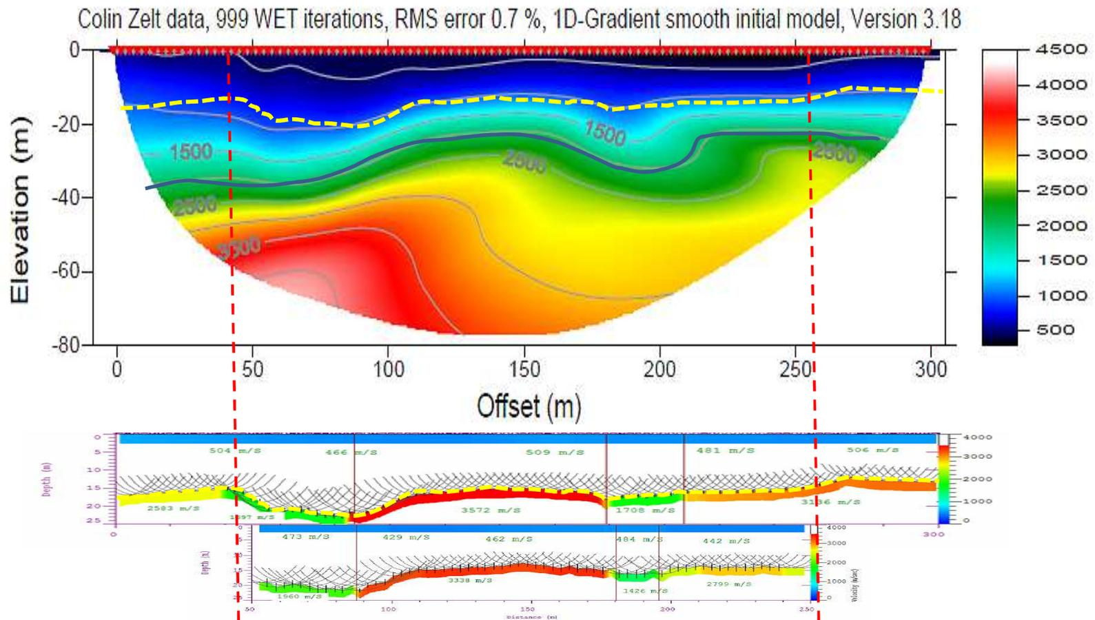
The 2000m/s contour is close to the actual bedrock surface which is interesting as this is what we normally use if there are unsaturated soils at the surface. The 2500 m/s contour is used in the marine environment . We then use the Reciprocal method to check bedrock velocities and ray tracing on interesting sections to check lower velocity zones
